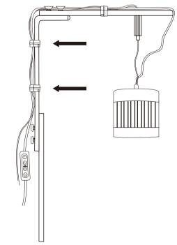
7) Connect the extension cable for the light and the extension cable for the power adapter.
