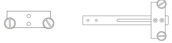
3) Connect ② bracket, align the gap of ② bracket with the screw holes of ① bracket, adjust the required length, and screw down with screws.
