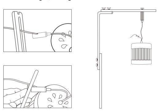
**6)** Run the wire around the bend of the bracket head and secure the wire and lamp wire with clamps.
